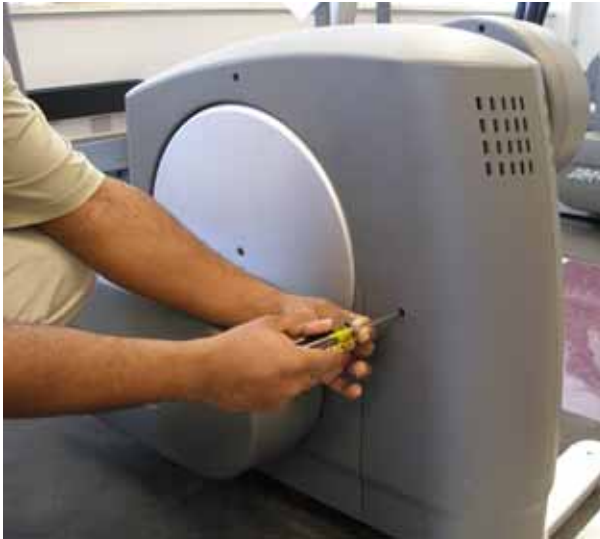
Fig. 1: loosening the main shroud screws
